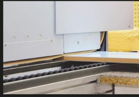
Preforming is a specific method of edge processing we offer at Teka Kitchen Gallery and done in our shop. In this method the surface material is formed and curved around the edge instead of just gluing an edge on the panel.
